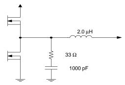
Figure 20. Filter Components
