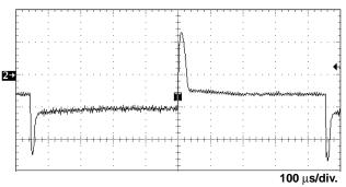
Trace 2- Regulator Output Voltage (output set for 1.55 V, 20 mV/div.)
