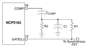
Figure 18. Small RC Filter Provides the Proper Voltage Ramp at the Beginning of each On–Time Cycle
