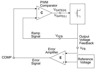
Figure 3. V<sup>2</sup> Control Diagram
