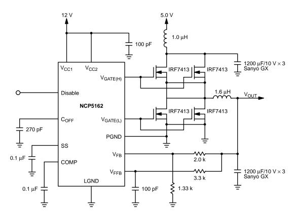
Figure 1. Application Diagram, 5.0 V to 2.5 V/20 A Core Logic Converter with 12 V Bias
